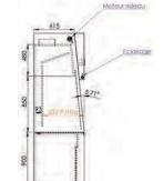
The BCS is an Extraction Fume Hood with vertical flow made in COPLAST. The fume hoods ensure the protection of the user and its environment thanks to a air negative pressure of the work area.
